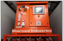
$SF_6$  Insulating Gas Processing – Sulfur hexafluoride gas or  $SF_6$  is used as an electrical insulation medium in many devices. Like oil-insulated equipment, the quality of the  $SF_6$  directly impacts the reliability and safety of the equipment. Shermco has mobile equipment that can reclaim and recycle your  $SF_6$  gas and return your equipment to service quickly and safely.
